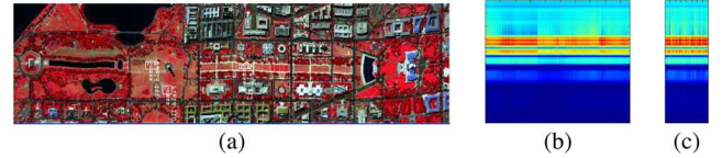
Fig. 11. (a) Simulated color IR view of an airborne hyperspectral data over the Washington DC Mall [37]. (b) Ground-truth pixel spectrum of grass pixels that are outlined with the white rectangles in (a). (c) Synthesized data spectrum using the Gaussian distribution.
