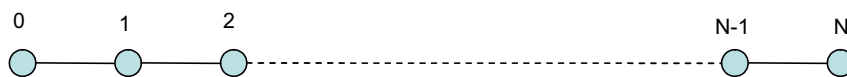
Fig. 17. Linear topology with nodes being reprogrammed using alternate mode of Stream with node 0 as the base node ( N = 1, 2, \dots, 11 ).
