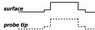
Figure 1: An illustration of a surface (solid line) and the trajectory followed by the probe tip (dashed line) when the surface is explored with a haptic device.
