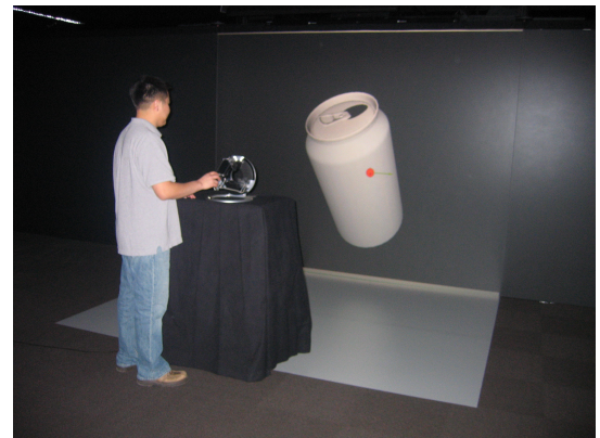
Fig. 3. A user feels a virtual can (with 43,539 vertices) displayed on a FLEX (CAVE™-like display from Fakespace Systems; www.fakesystems.com ) using the Purdue Portable Haptic Display. The force-feedback device (Omega device) is controlled by a laptop mounted inside the cart. The laptop transmits visual information via wireless network to a computer (not shown) operating the FLEX.
