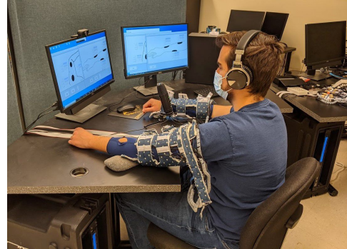
Fig. 1. Photo of a participant wearing one tactile display on the upper left arm and the other on the right forearm. The computer screen shows a diagram of factors on the attended arm(s), with three buttons representing the three frequency conditions at each location. The participant selected the response by clicking on the button corresponding to the location and frequency combination with the right hand.
