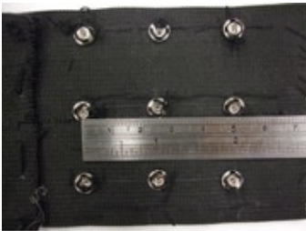
Fig. 1. The 3x3 tactor array with an inter-element spacing of 25mm
