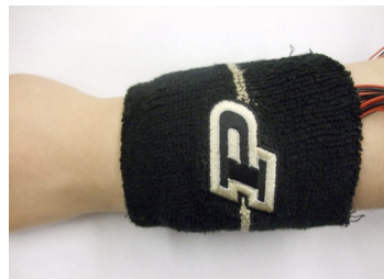
Fig. 2. The wristband for ensuring contact between the tactors and skin
