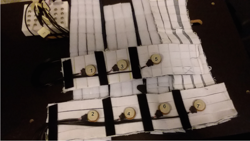
Fig. 1. Layout of factors for the 7-channel tactile aid to lipreading.
