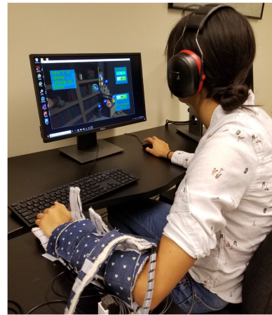
Fig. 1. Experimental setup with the phonemic-based speech communication system TAPS (TActile Phonemic Sleeve).
