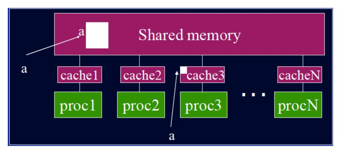
Two issues, coherence and consistency. *Coherence*: Behavior of the memory system when a single address is accessed by multiple threads. *Consistency*: Orderings of accesses to different addresses by multiple threads.
