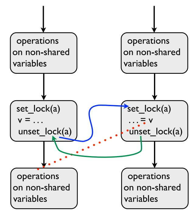
The OpenMP standard requires that OpenMP fences on Power processors wait until new value visible to all and old values invalidated 42
