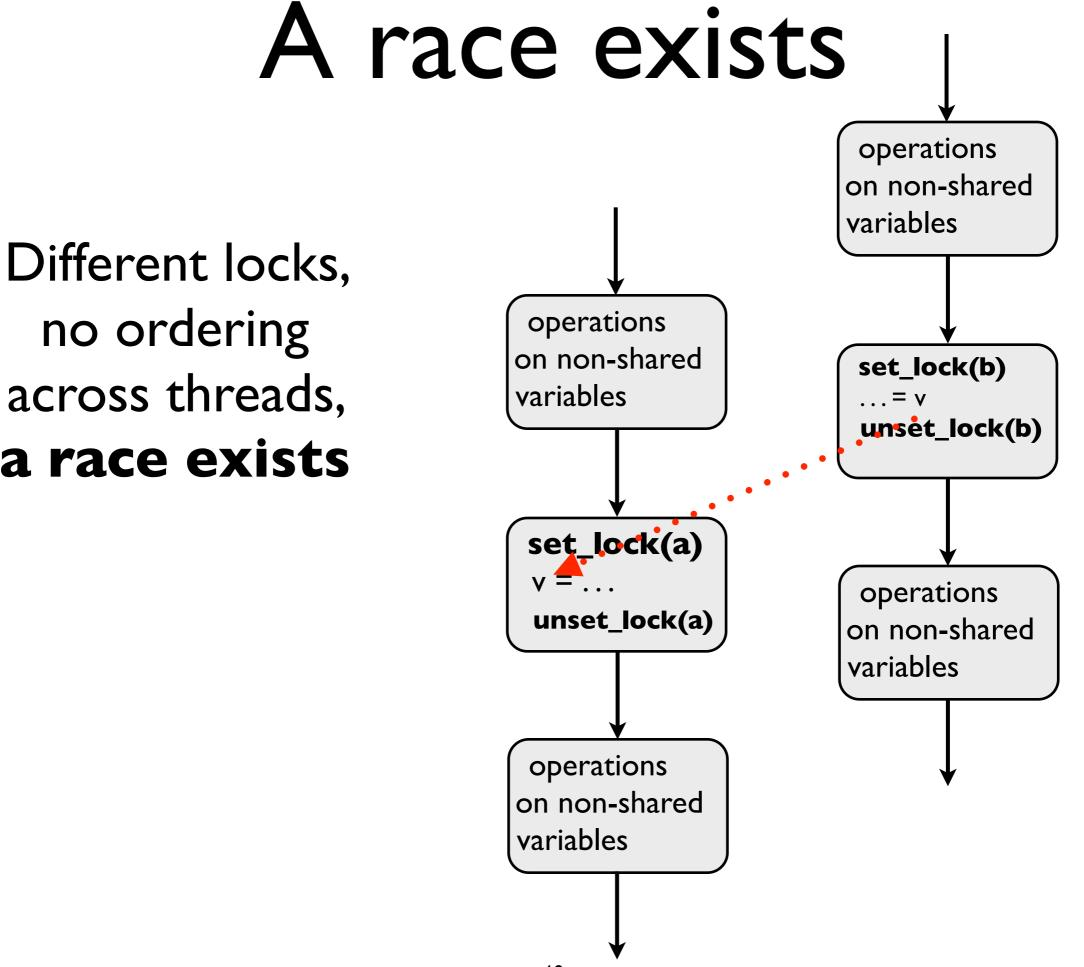
no ordering across threads, a race exists For an order to exist between v= and =v it must be that the *fence* in the unset\_lock() forces any new value of v out before the unset\_lock completes
