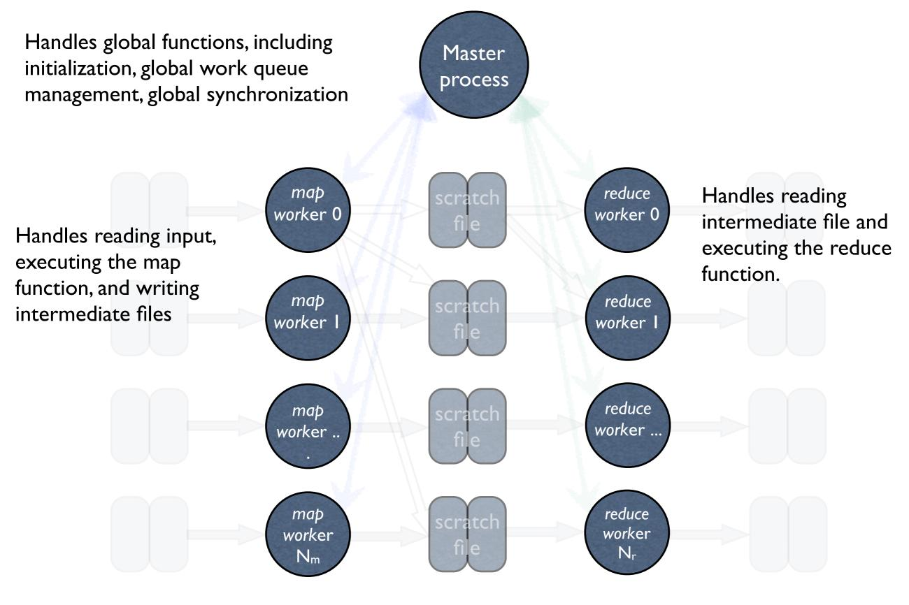
Intermediate files allow buffered high volume communication between mappers and reducers
