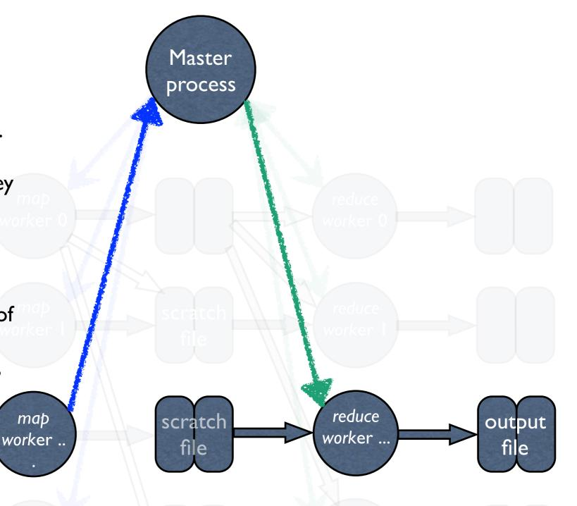
The master process will use the scheme to map keys (I'll call it the hash function). The hash function will map all keys onto  $k_{ReduceFiles}*|reducers|$  different files. When a reducer is ready for work, it will give one of the  $k_{ReduceFiles}*|reducers|$  different sets of file files to that reducer. When all those files are consumed, the reducer can ask for another file.
