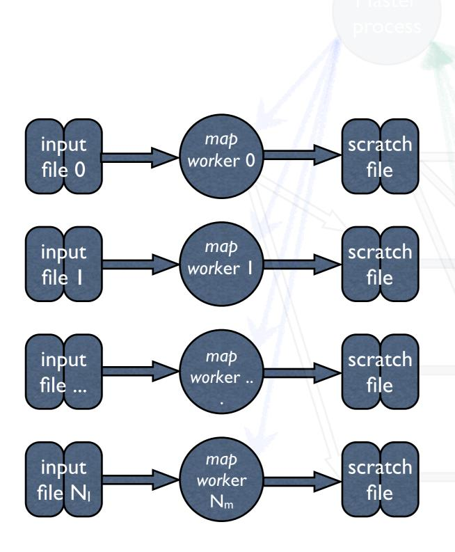
We also do not want one file created by each map process for each reduce process (i.e. approximately [*keys*//*reducers*]] keys per file. Would be bad for load balancing purposes.
