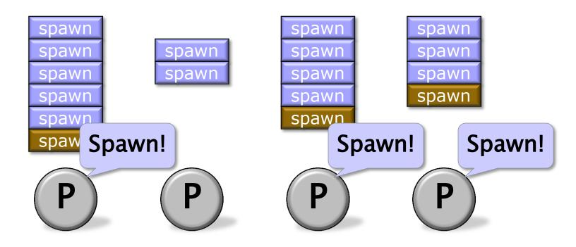
When each processor has work to do, a spawn is roughly the cost of about 25 function calls.
