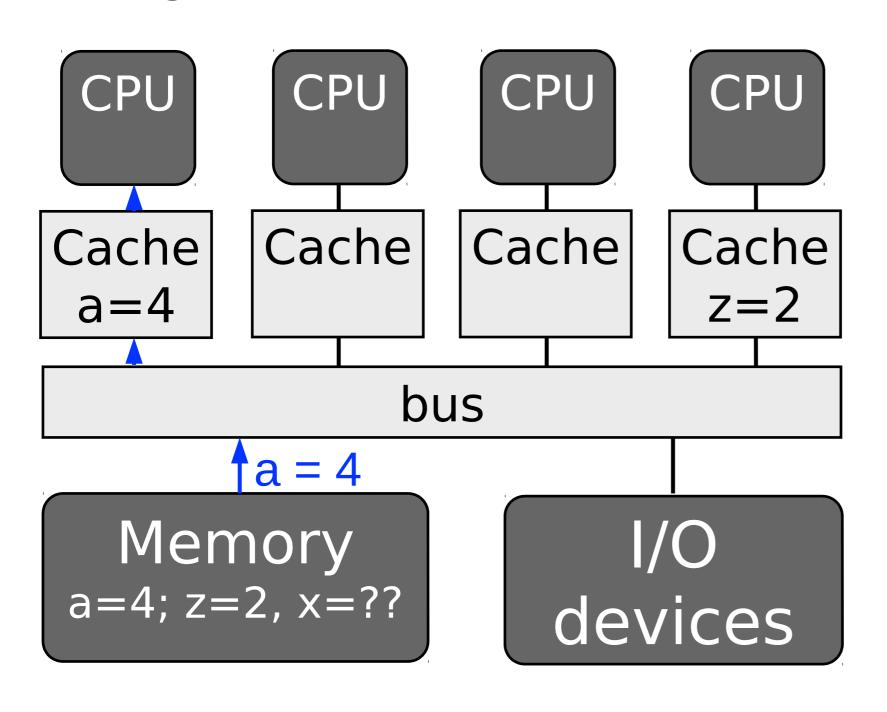
T0: z = a load reg2, from (a) // load a from memory st reg2, into (z)
