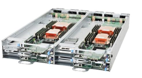
A node is one or more processors along with associated devices (disk drive, memory, i/o cards, communication cards, etc.
