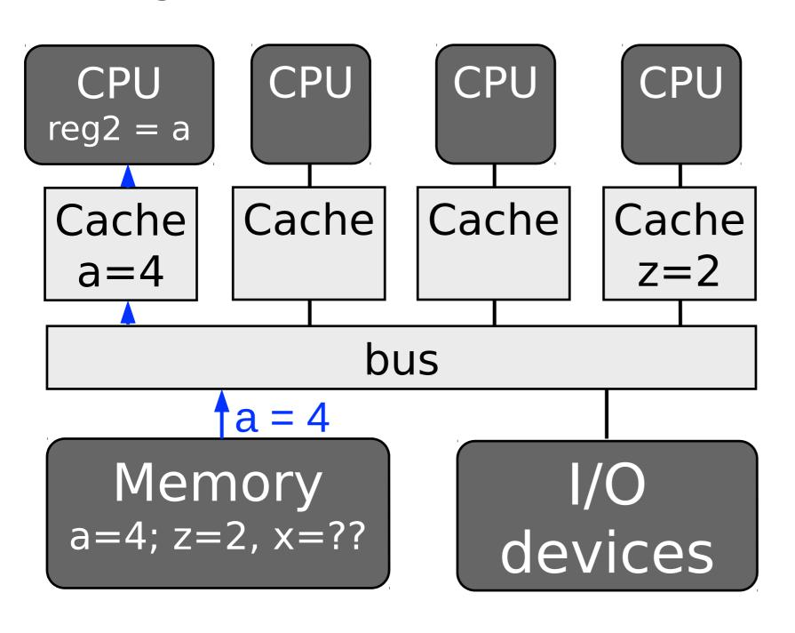
T0: z = a load reg2, from (a) // load a from memory st reg2, into (z) // reg2
