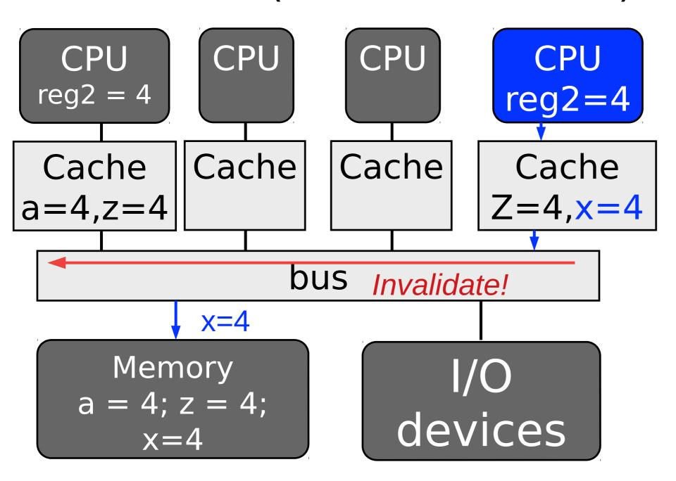
Hardware makes sure a core/processor reads the latest value assigned to memory (cache coherence)
