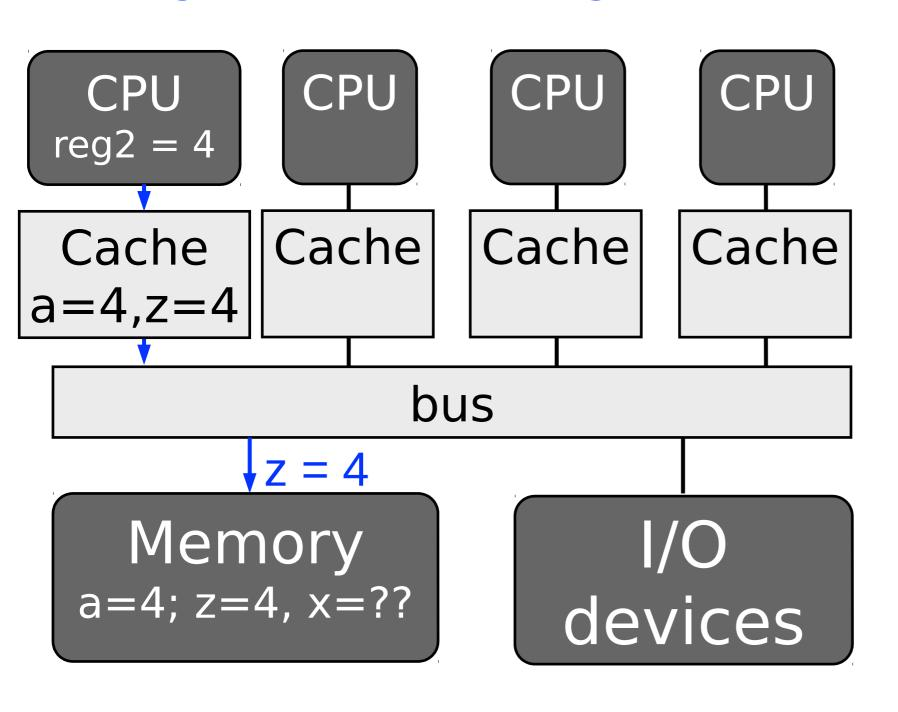
Tn: x = z // instruction in rightmost CPU load reg2, from (z) st reg2, into (x)
