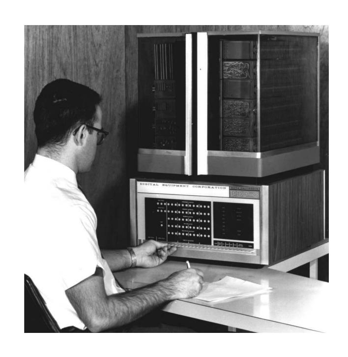
A Digital Equipment Corporation *PDP-8* (programmable data processor)
