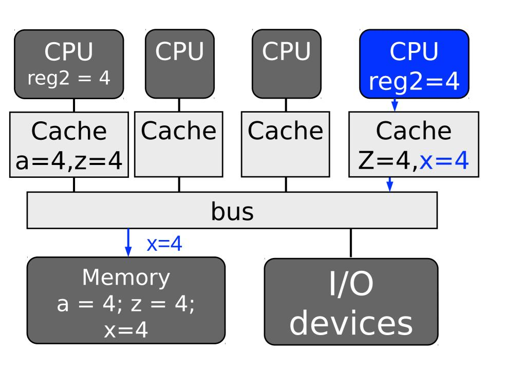
Tn: x = z // instruction in rightmost CPU load reg2, from (z) st reg2, into (x)
