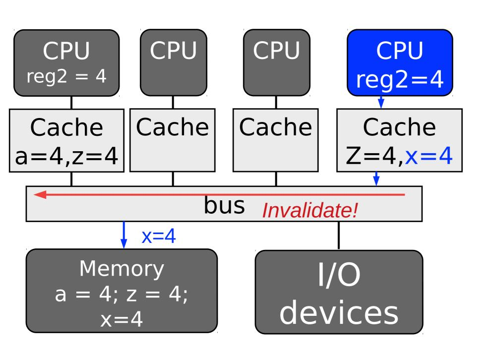
Hardware makes sure a core/processor reads the latest value assigned to memory (cache coherence)
