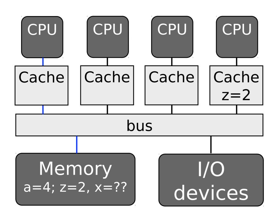
T0: z = a load reg2, from (a) // load a from memory st reg2, into (z)
