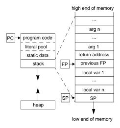
Figure 1: The memory layout of a stack frame after a function has been called.
